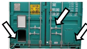
Figure 9.12 Dry bulk discharge hatch (rear)
