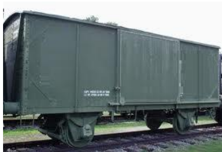
Figure 9.3 Sliding door (Rail Wagon)
