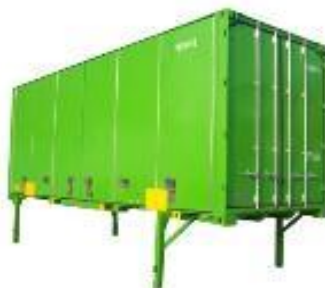
Figure 3.67 – Class C side door swap body
