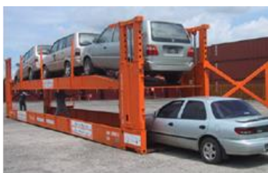
Figure 3.54 – 45-foot car carrying folding flatrack
