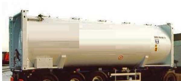
Figure 3.69 – 30-foot stackable swap tank for powder
