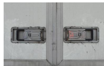
Figure 9.7 Recessed handled with protruding eyes
