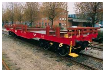
Figure 3.96 – Special flat wagon
