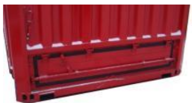
Figure 3.43 – Letterbox type hatch in container front wall
