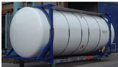
Figure 3.68 – Swap tank showing exposed ends
