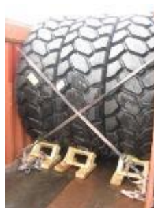
Figure 3.23 – 20-foot open top with extra large tyres
