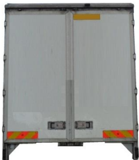
Figure 9.2 Swing door (Road vehicle)
