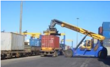
Figure 3.88 – Container loading using reach stacker
