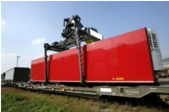
Figure 3.87 – Trailer1 loading using grapple arms
