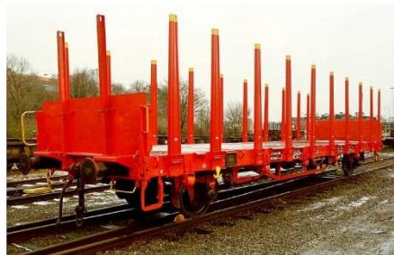
Figure 3.92 – 2 axle flat wagon
