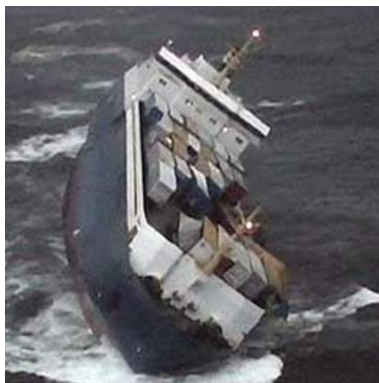
Figure 1.5 – Heavily listing ship after cargo has shifted
