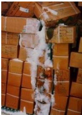
Figure 1.12 – Ice from leak in door gasket
